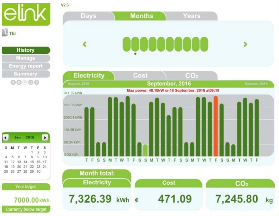
Fig. 4 Monthly electrical consumption of 2 nd power supply
