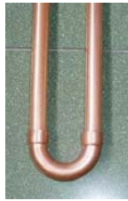
Fig. 2 Connection point of the U-shape receiver tube
