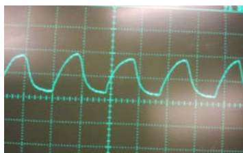
Fig. 6 Typical recordings from thermistor indicating breathing rate, and the inhalation and exhalation activity are traced from the slope of the increase and decrease of the curves
