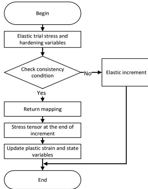
Fig. 2 Flowchart of implicit elastic predictor/return mapping algorithm
