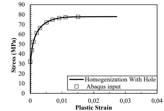
Fig. 14 Validation of the homogenization material properties with input data
