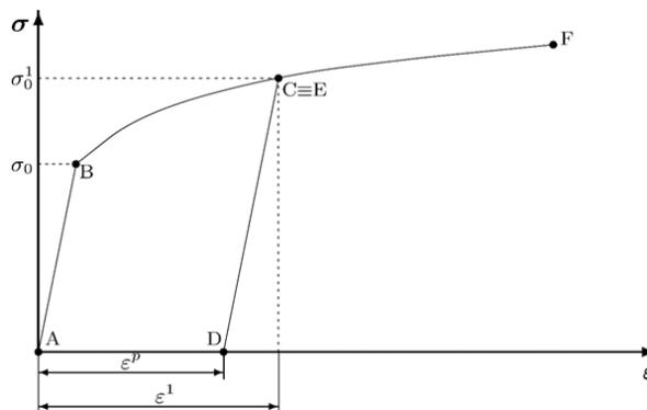
Fig. 1 Mathematical model of uniaxial tensile test
