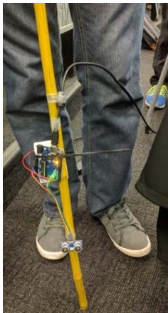
Fig. 2 Example of an interactive walking cane for blind people made by one of the teams
