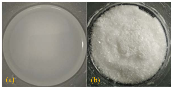
Fig. 1 Samples of (a) alumina gel (b) alumina aerogel
