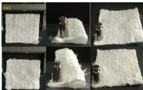
Fig. 7 (a) Nanoporous Al 2 O 3 aerogel composites prepared by particle method (left: original sample; middle: compressed sample; right: recovery sample), (b) Aluminum-silicon aerogel composites with reinforcement phase of mullite fibers (left: original sample; middle: compressed sample; right: recovery sample)
