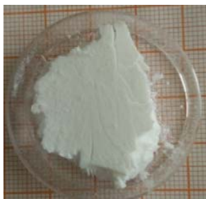
Fig. 4 The sample of aluminum-silicon aerogel
