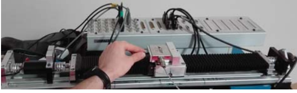
Fig. 7 Co-manipulation experiments, the operator apply a specific force on the force sensor of the robot presented into Fig. 1
