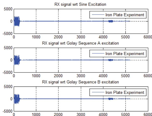
Fig. 12 The received echoes coming from the iron plate with respect to different excitation signals at 64<sup>th</sup> channel
