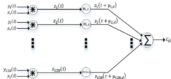
Fig. 1 Block Diagram of a Correlation Based Beamformer
