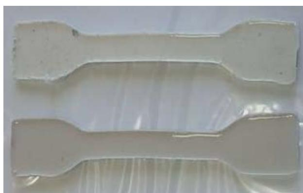
Fig. 6 Moulded Ag doped CNFs/RTV664 composite
