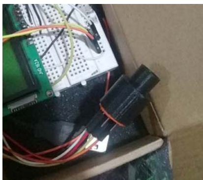
Fig. 3 Mouthpiece with MQ 138 sensor
