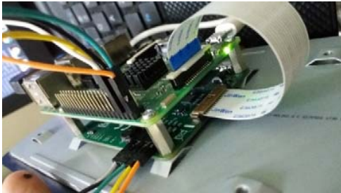
Fig. 4 Raspberry Pi display connection
