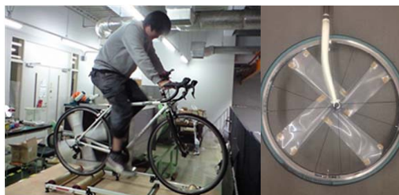
Fig. 1 Bicycle with Wells turbine in wheels
