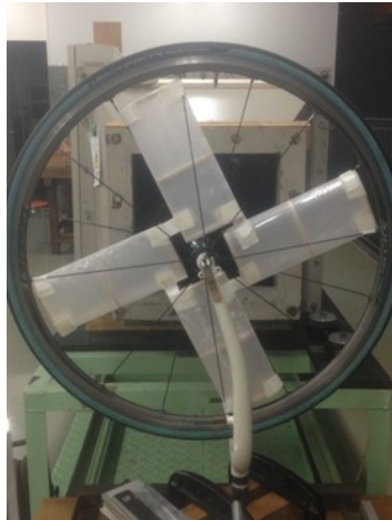
Fig. 3 Wells turbine in a wheel
