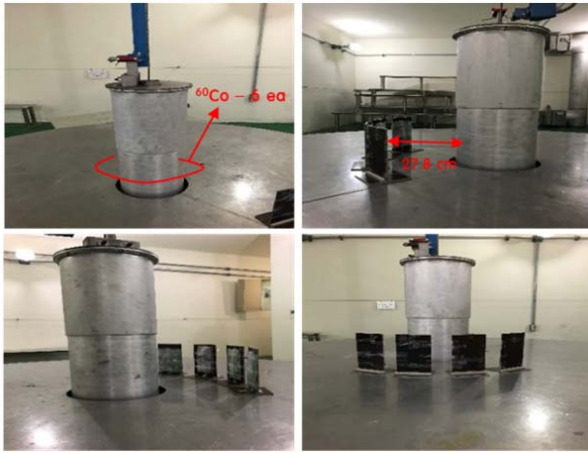
Fig. 2 Experimental set-up of gamma-ray irradiation of NPT-IGBTs
