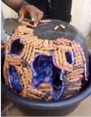
Fig. 9 Arranging and gluing the clay pieces to cover the plastic surface
