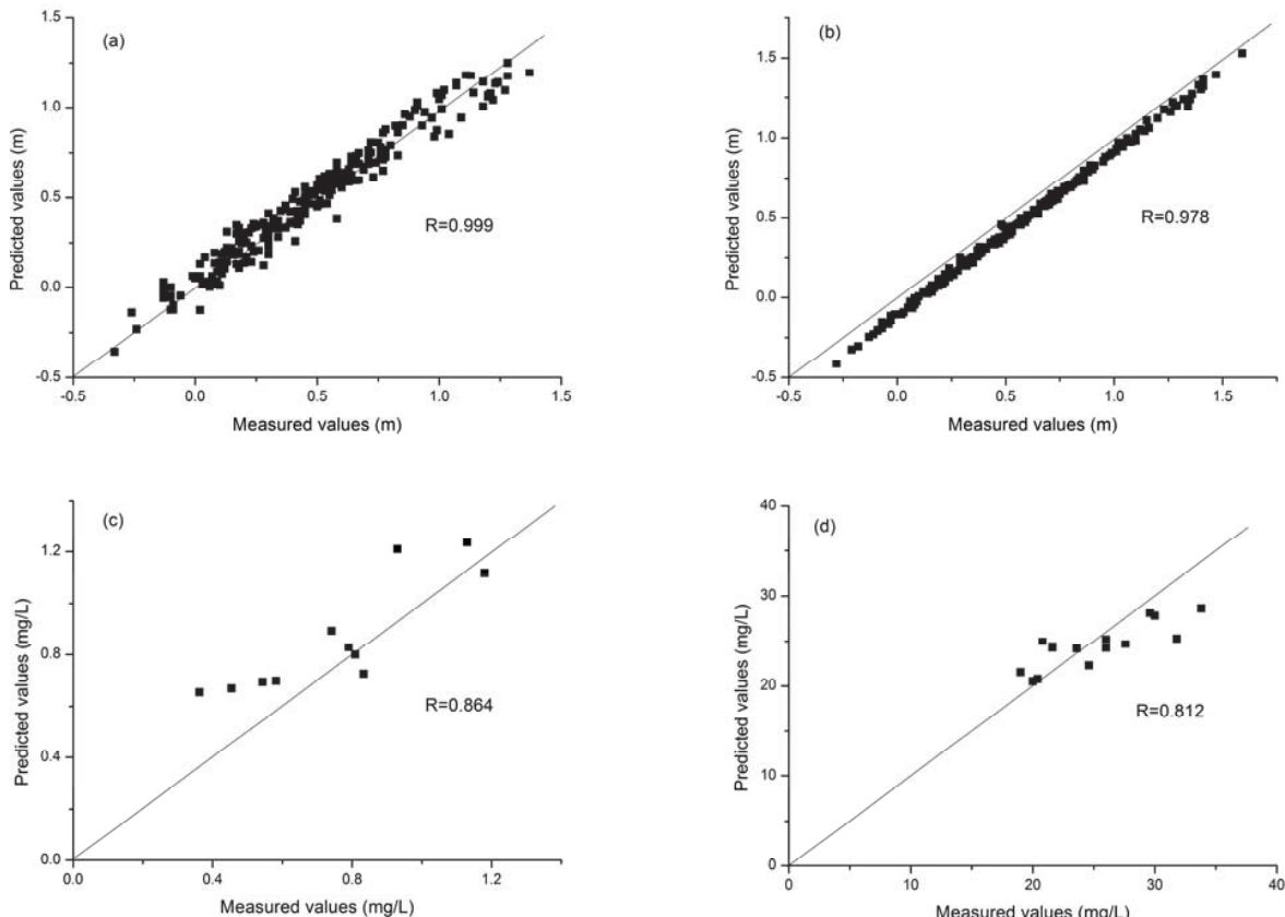
Fig. 3 Correlation between measured and simulated values: (a) water level in Heshun Site; (b) water level in Jietou Site; (c)  $\text{NH}_3\text{-N}$  concentration in Xiangling Site; (d) COD concentration in Jietou Site
