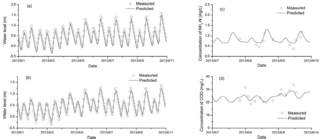
Fig. 2 Comparison between measured and simulated values: (a) water level in Heshun Site; (b) water level in Jietou Site; (c) NH<sub>3</sub>-N concentration in Xiangling Site; (d) COD concentration in Jietou Site
