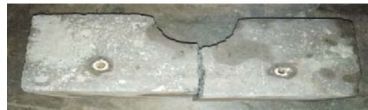
Fig. 7 Concrete block after flexural strength
