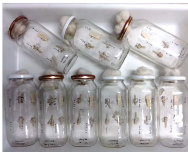
Fig. 19 Screening fungal test devices (ex: PP) for Wood Polymer Composite samples and pine wood controls
