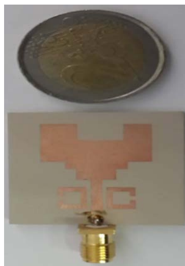
Fig. 7 Fabricated prototype of the proposed antenna
