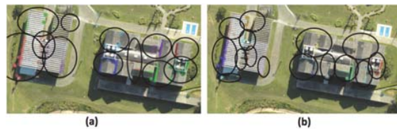
Fig. 7 Landmark Selection for the Aerial Mosaic using ORB. (a) is the Result for the X-Means in [22] and (b) is the result for the Proposed X-Means
