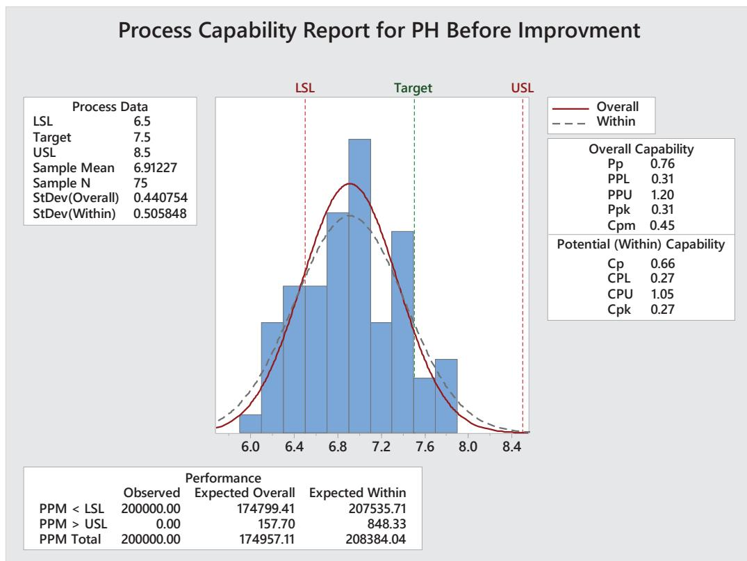
Fig. 5 Process Capability of pH (Before Improvement)
