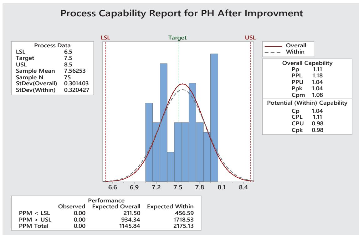
Fig. 7 Process Capability of pH (After Improvement)
