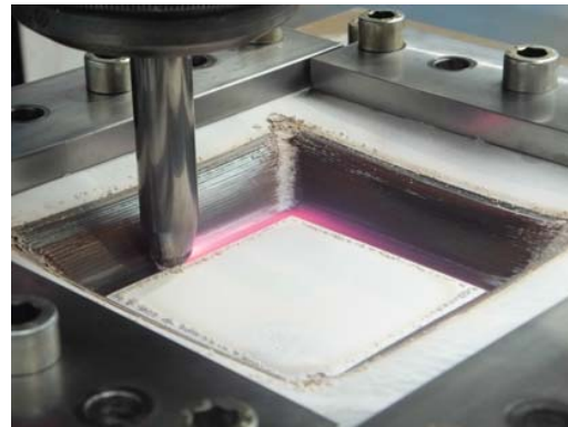
Fig. 3 IASPIF process during pyramid profile forming and induction heating
