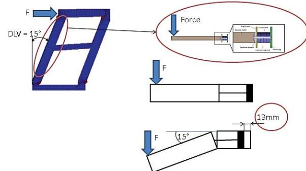
Fig. 12 Limitation of bending crash box at DLV of cab frame
