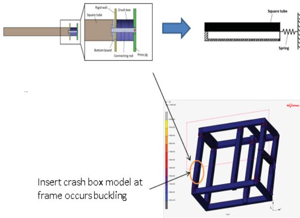
Fig. 4 Install absorption part at cab frame
