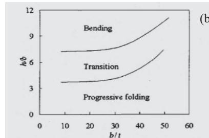
Fig. 3 (a) Stress-strain curve of deformation mode, and (b) Deformation mode mapping, cited from Shinohara et al. [18]
