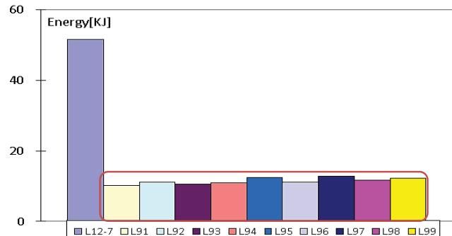
Fig. 7 Comparison of energy absorption between (L12-7) and improvement bending-compress
