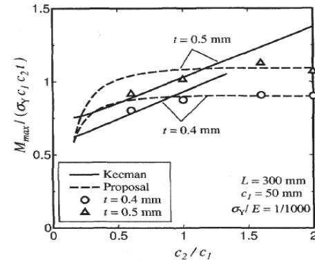
Fig. 2 Comparison between Kecman's theory and FE analysis. Cited from Masuda et al. [17]
