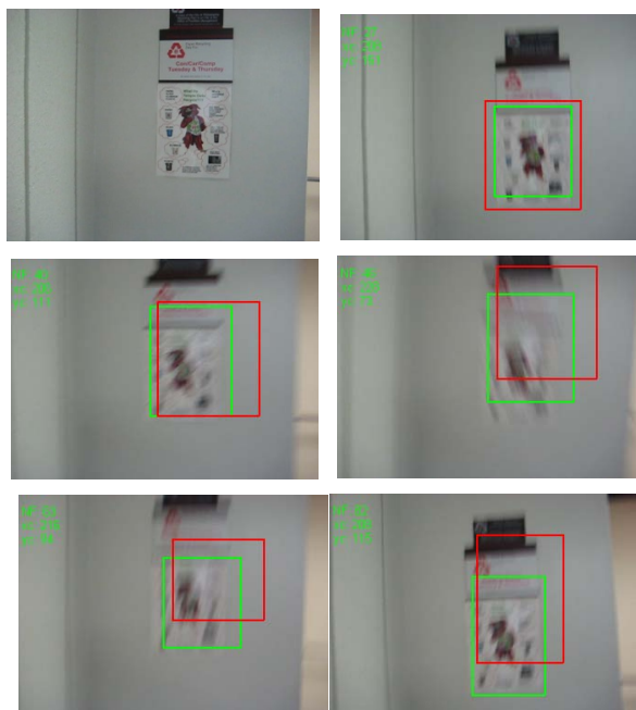
Fig. 6 The tracking result of selected target for frames 1, 27, 40, 47, 63, and 82 of blur owl
