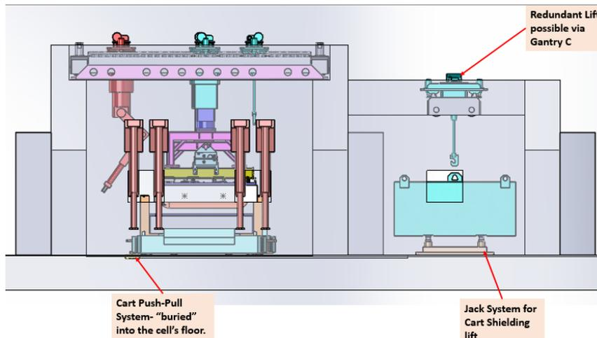
Fig. 13 Side View- BB Assembly Cell Transparent Walls
