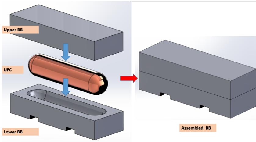
Fig. 9 Graphical Explanation of the BB Assembly
