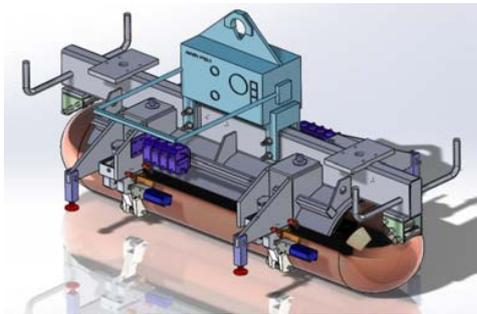
Fig. 6 Vacuum Lifter for UFC (safety fingers active)
