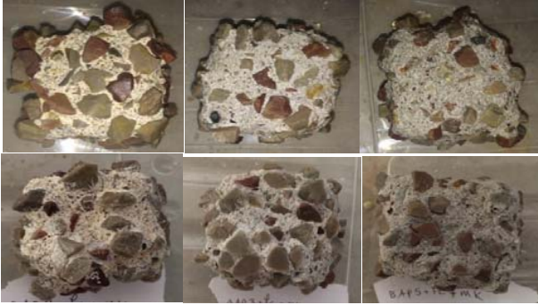
Fig. 5 The visual appearances of specimens after 8 weeks exposure to sulfuric acid solution at age of 90 days of cure
