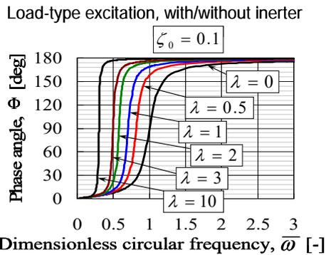
Fig. 12 Variation of the phase angle versus the dimensionless circular frequency, obtained under load-type excitation in the presence and absence of the inerter, for a fixed value of the damping ratio
