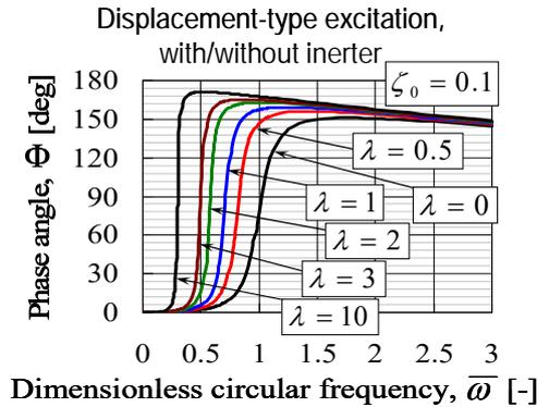
Fig. 22 Variation of the phase angle versus the dimensionless circular frequency, obtained under displacement-type excitation in the presence and absence of the inerter, for fixed damping ratio
