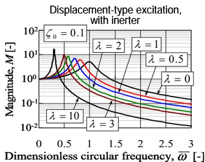
Fig. 18 Variation of the magnitude versus the dimensionless circular frequency, obtained under displacement-type excitation in the presence and absence of the inerter, for fixed damping ratio
