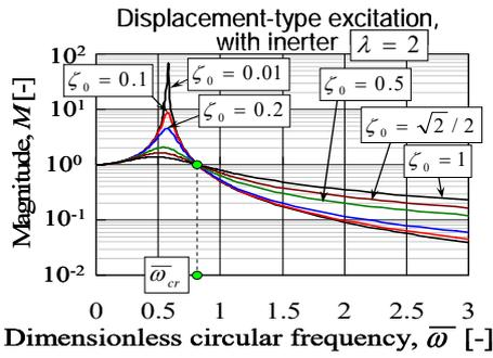
Fig. 17 Variation of the magnitude versus the dimensionless circular frequency, obtained under displacement-type excitation in the presence of the inerter, for various values of the damping ratio
