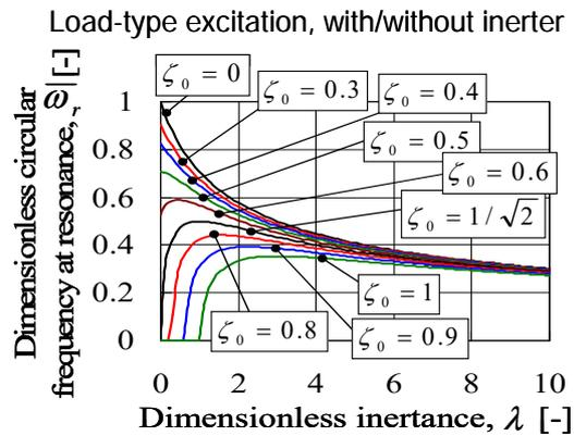
Fig. 6 Variation of the dimensionless circular frequency at resonance versus the dimensionless inductance, for various damping ratios
