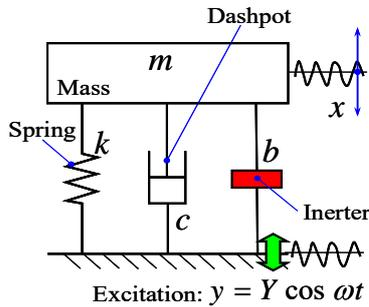
Fig. 2 Schematic view of the damped 1DOFS under displacement-type excitation, in which the mass element is supported by an elastic element, connected in parallel with a dissipative element and an inerter
