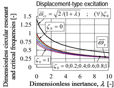
Fig. 19 Variation of the dimensionless circular frequency at resonance, and dimensionless circular critical frequency versus the dimensionless inductance, for various values of the damping ratios
