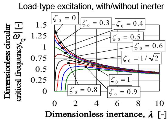
Fig. 7 Variation of the dimensionless circular critical frequency versus the dimensionless inductance, for various values of the damping ratio
