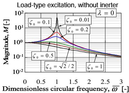
Fig. 3 Variation of the magnitude versus the dimensionless circular frequency, obtained under load-type excitation in the absence of the inerter, for various values of the damping ratio
