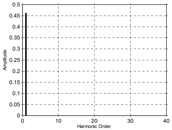
(c) Line current spectrum of phase a
