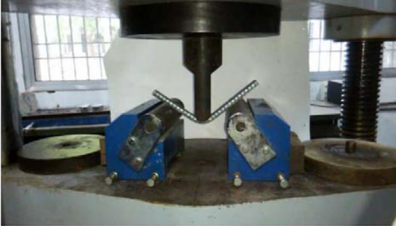
Fig. 2 (A) Experimental setup on universal testing machine
