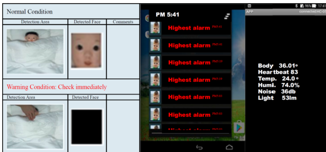
Fig. 5 Example of emergency alarm condition
