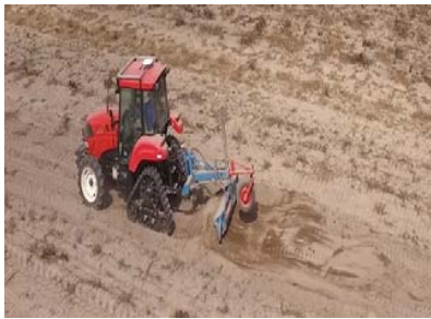
Fig. 8 Building bumps and hollows using a plough
