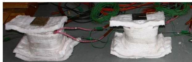
Fig. 2 HFRC specimens during the heat treatment
