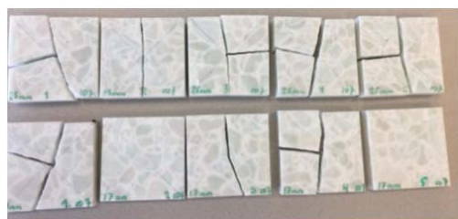
Fig. 5 Results of 10-J impact event. (first row: 0.017 mm thickness, second row: 0.025mm thickness)
