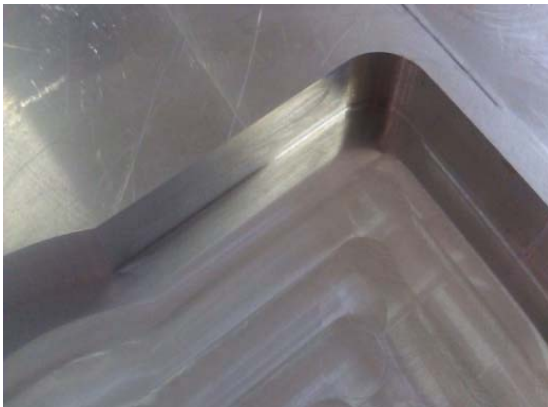
Fig. 10 Warm Cast after Machining
