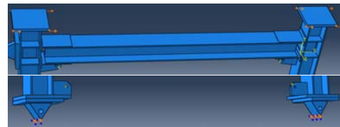
Fig. 2 Conditions of supports
