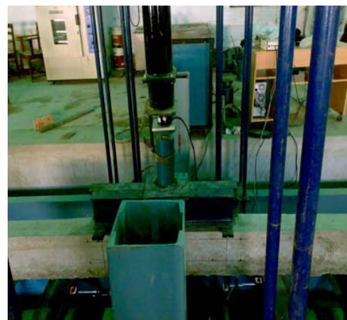
Fig. 7 Arrangement for flexural testing in Load Frame
