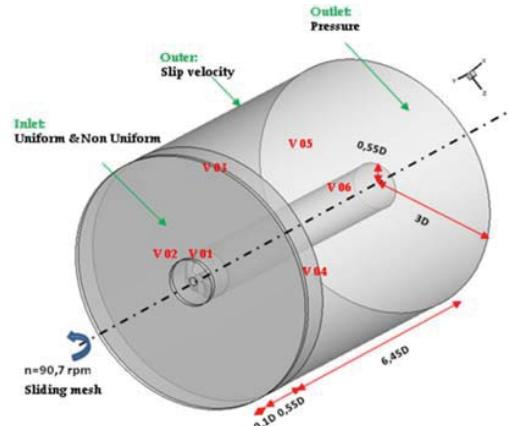
Fig. 6 Computational domain for unsteady simulation, for HSP Seiun Maru propeller
