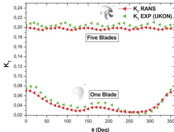
Fig. 11 Thrust coefficient for Sieun Maru HSP during one revolution
