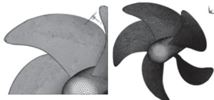
Fig. 3 Propeller surface mesh
