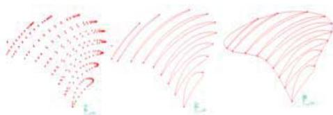
Fig. 2 The propeller drawing steps
