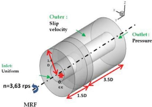
Fig. 4 Computational domain for steady simulation
