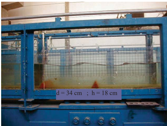
Fig. 16 Free-surface waves over two obstacles
