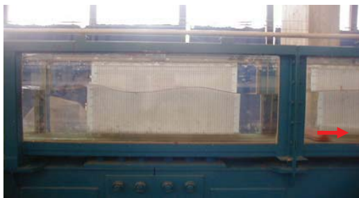
Fig. 11 Free-surface standing gravity waves
