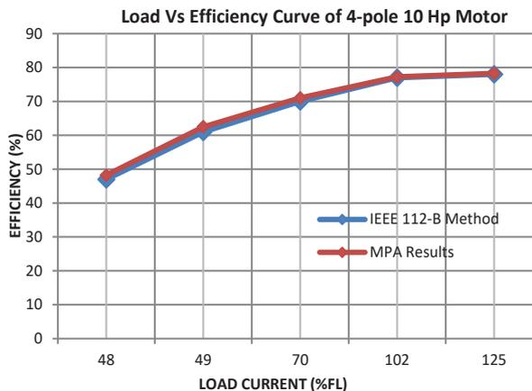
Fig. 10 Comparison of the Performance on 10 HP Motor
