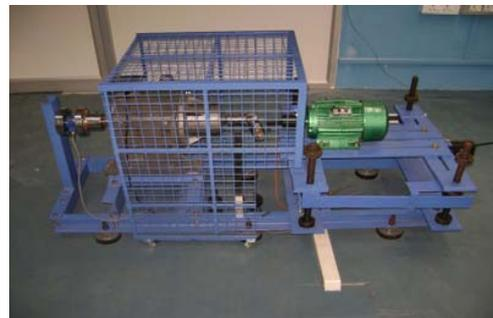
Fig. 7 View of the Motor Test Bed - 1 with 5 HP Motor installed
