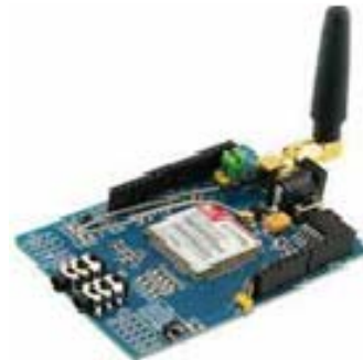
Fig. 8 Arduino shields for GSM mobile communication
