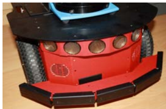
Fig. 3 Pioneer P3DX fitted with the Polaroid Sonar Array (front and rear) and a Bumper Array at the front
