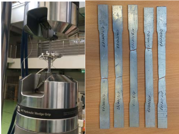
Fig. 2 Laboratory stand and specimens used to determine strength characteristics of steel
