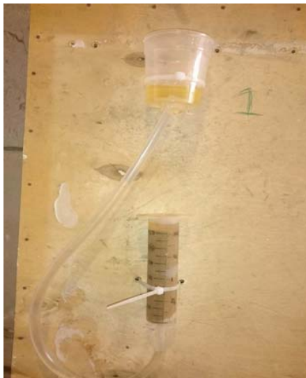
Fig. 7 Addition and drainage of the reactant into the MICP-Treated sand sample
