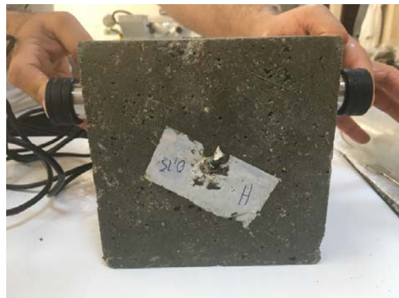
Fig. 2 UPV Testing System
