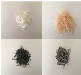
Fig. 1 Synthetic and steel fibers
