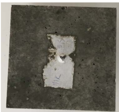
Fig. 5 Cube specimens before compressive strength test
