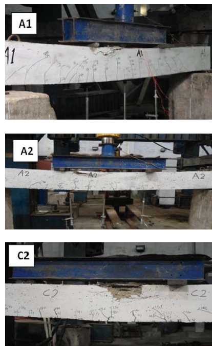
Fig. 6 Cracks Patterns of beams A1, A2, and C2 at failure
