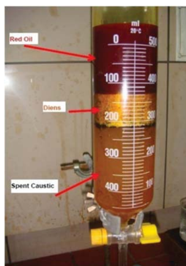
Fig. 1 Separated phases in the tower output sample
