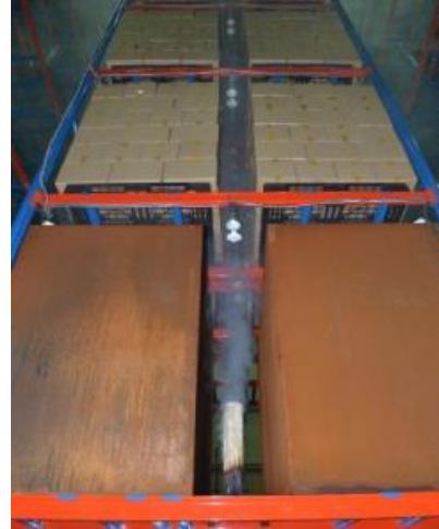
Fig. 4 Smoke flow by cotton fire
