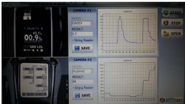
Fig. 11 Measured concentrations for testing two gas leakage detectors (150 seconds)
