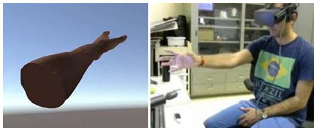
Fig. 2 ARWED system where the subject's right hand is mapped to the virtual left hand
