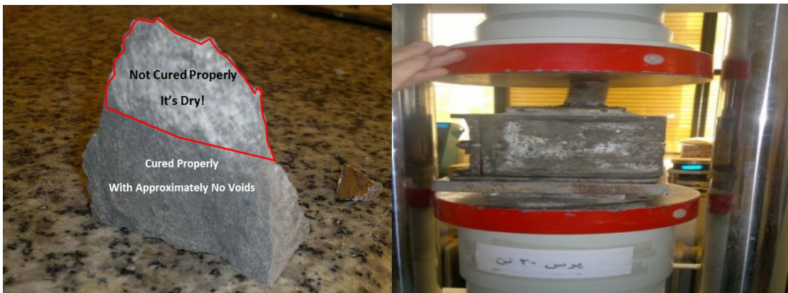
Fig. 4 Pressing the Samples by Applying 20 MPa
