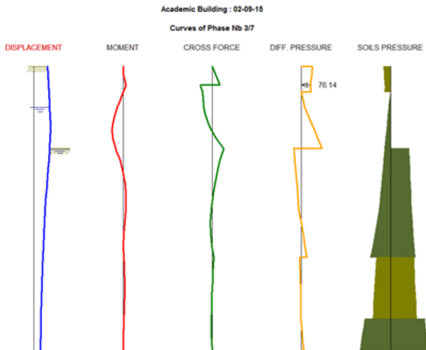
Fig. 10 Excavation to the second layer
